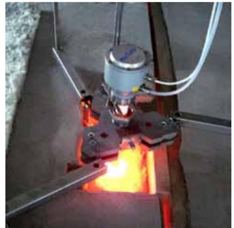
Installed sensor with the Mounting and Holding Device
