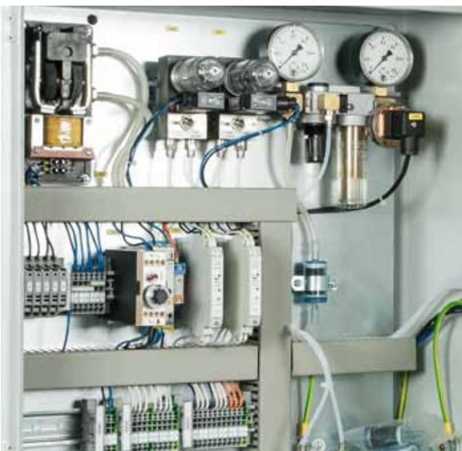
Reference Air Unit with pressure control valve and Air Pulsing Unit
