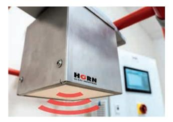
A special ceramic sealing plate on the measuring aperture ensures that radar waves can penetrate it, but no exhaust gases can escape. Consequently, no condensates can settle on the radar sensor. Maintenance work is reduced.
