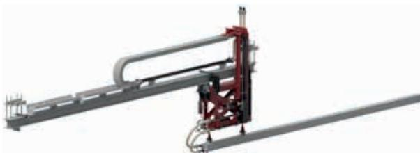
The HORN® entrance cooler of Type HECO, which is installed in the entrance section of the tin bath, provides optimum production conditions in the tin bath right from the start. The cooling element is positioned above the glass ribbon and absorbs heat radiation from it in order to ensure the perfect glass temperature for the forming process (between 950 °C and 840 °C).
