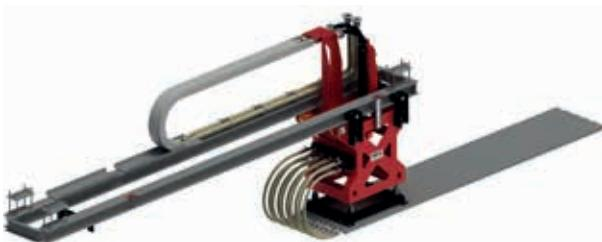
The exit end cooler of Type HEECO, which is installed in the narrow part of the tin bath, serves to cool down the glass ribbon to the optimal lift-out temperature (approx. 610 °C), which is crucial for ensuring smooth production.
