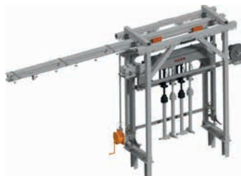
A swing-out mechanism is available in order to simplify maintenance work.
