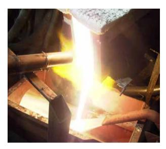
Finally, the HORN® service company heats up the furnace to operation temperature with special heat-up burners and measurement equipment to ensure the proper temperature gradient and controlled expansion of all refractory material.
